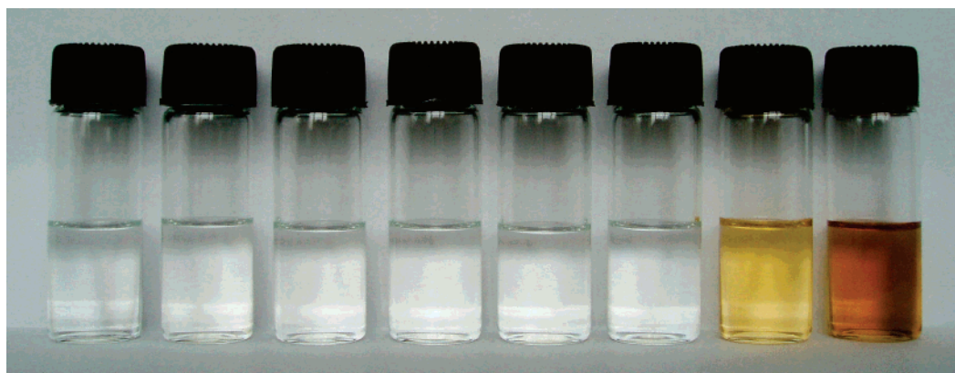
Figure 5. Color changes of P3 ( 5\ \mu\text{M} ) in chloroform upon addition of no anion, \text{Cl}^- , \text{Br}^- , \text{I}^- , \text{BF}_4^- , \text{PF}_6^- , \text{H}_2\text{PO}_4^- , and \text{F}^- (from left to right) with the concentration of 10^{-4} M.
